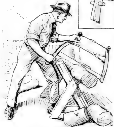
A simple peg makes the task of sawing wood a little less strenuous
